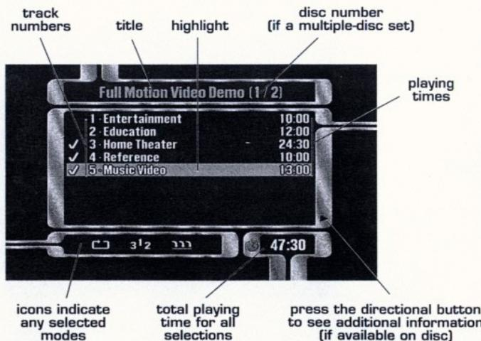
To see current disc information during play, press Select. The status display appears over the video image, showing the current track number, elapsed and remaining time for the track and the disc, and icons for any selected modes (repeat, shuffle, or sample).
