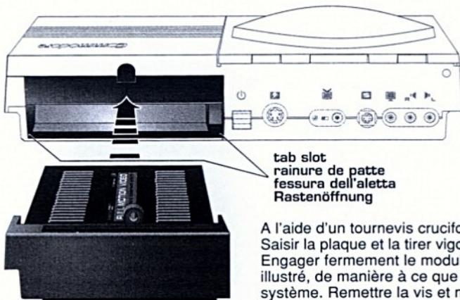
Using a Phillips-head screwdriver, remove the screw on the plain back plate. Grasp the plate and pull firmly to release the internal tabs. Press the Full Motion Video Module solidly into the case, as illustrated, until the screw hole is flush with the back of the system. Replace the screw and discard the old plate.
