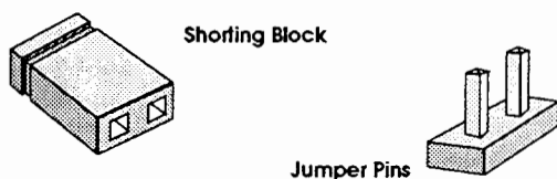
Figure 2.1 – Jumper block and pins.
