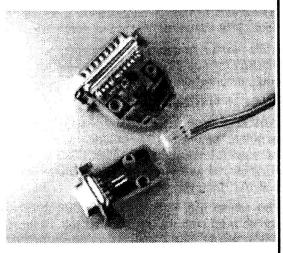
If you have an additional disc drive fitted to your AMIGA, then simply plug this new lead into its own 'daisy chain' socket.
