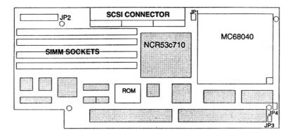
3. Set the chip down on the socket. When you have determined that all of the pins are resting in their socket holes, press the chip firmly down in the socket.
