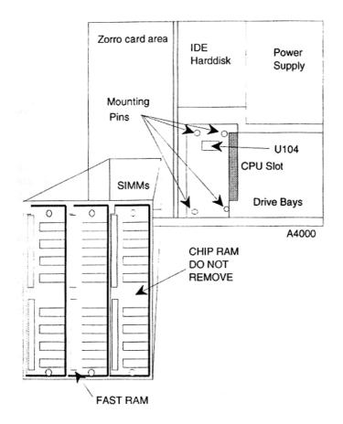
The SIMMs are located on the lower left of the motherboard. You will have to remove any expansion cards to see the SIMMs.
